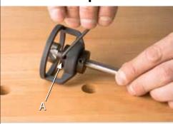
Slide the completed assembly over the top of your bit shank to the desired depth and secure the bottom stop collar (A) in place with the allen wrench.
