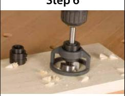
Insert your bit and the assembled depth stop into your drill chuck, secure and begin drilling perfect flat bottom holes at the perfect depth.
